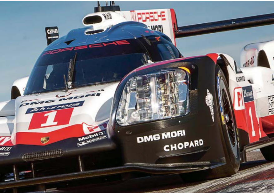
Each headlight has twelve pairs of LEDs and reflectors.
