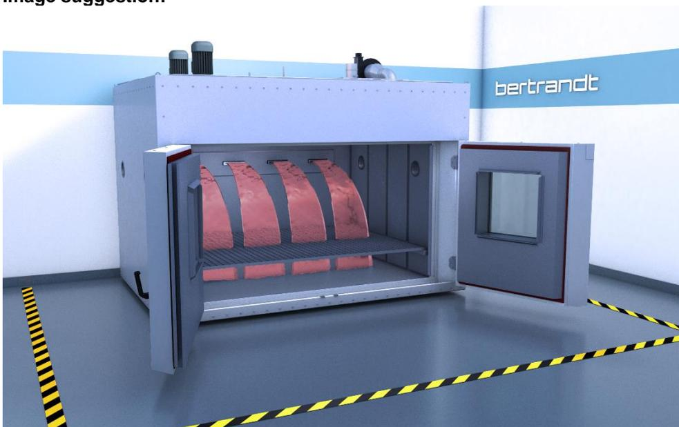
BU: The splash water test chamber can be used to validate electronic components.
