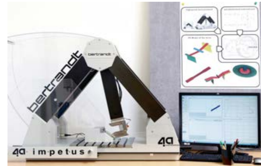
4a impetus: a complete system for generating valid material data for simulation purposes.
