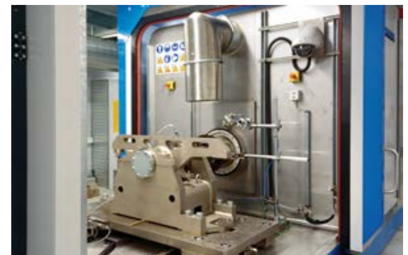
On the new inertia brake dynamometer, disk brakes are exposed to the same stresses as in road use.
