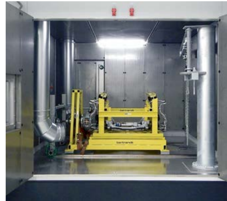
A complete front axle is installed ready for testing in the new test chamber.
