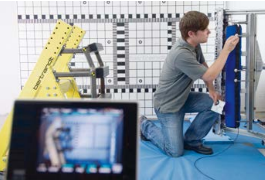
FlexPli, the new impactor, is already in use in our test laboratory.
