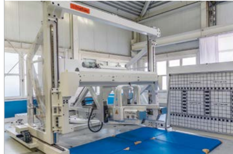
New test laboratory for evaluating pedestrian safety and misuse requirements for sensor systems.
