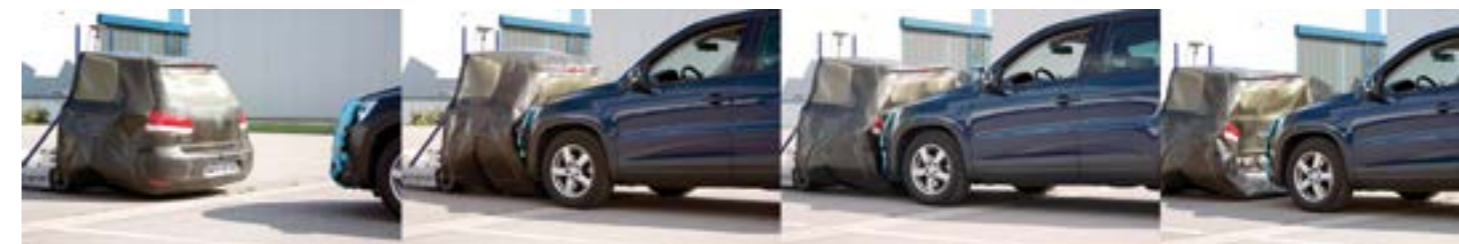
"Tail end of traffic jam" scenario: test procedure with pre-formed target.
