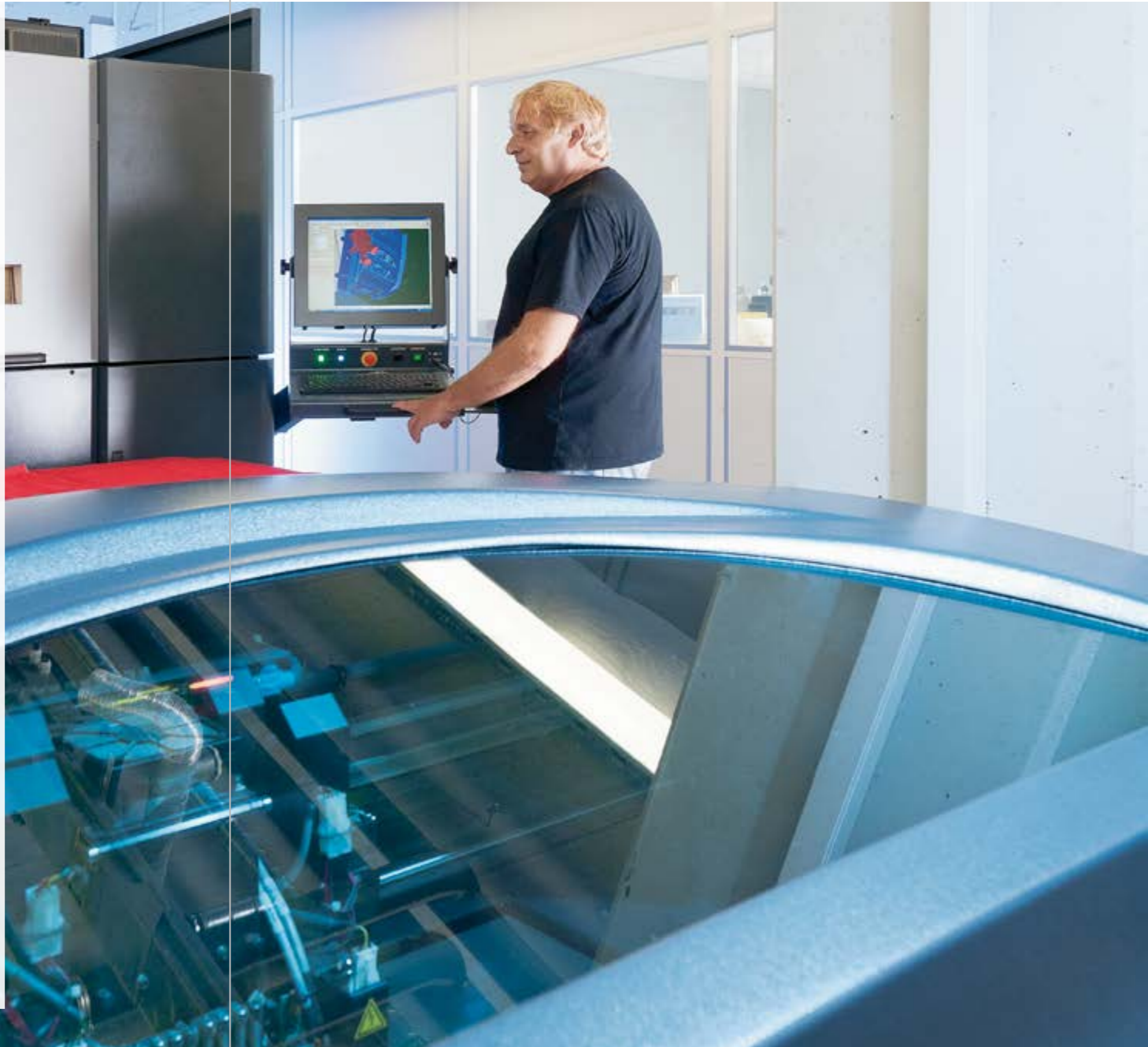
Milling injection moulding tools using state-of-the-art equipment: the DMU 105.
