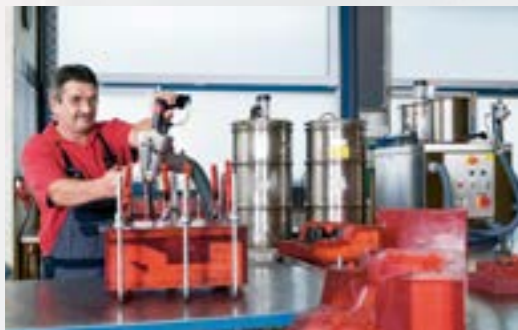
Low-pressure RIM systems: developing parts for simple function testing using non-production materials.
