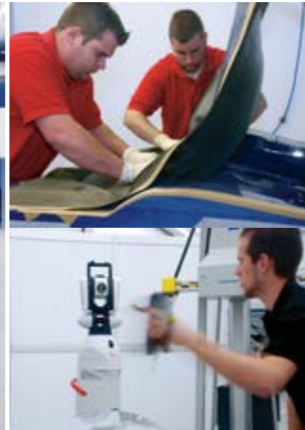
▲ Laminating with CFRP. ▲ Measuring with the laser tracker.
