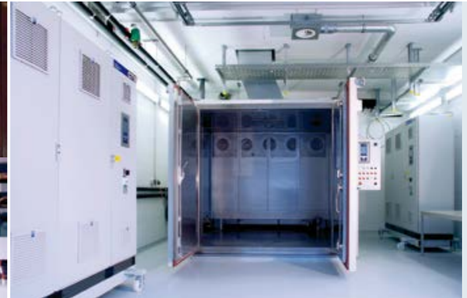
▲ Climate chamber in the battery test centre.
