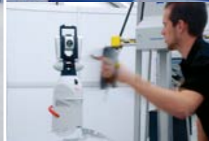
▲ Laminating with CFRP. ▲ Measuring with the laser tracker.
