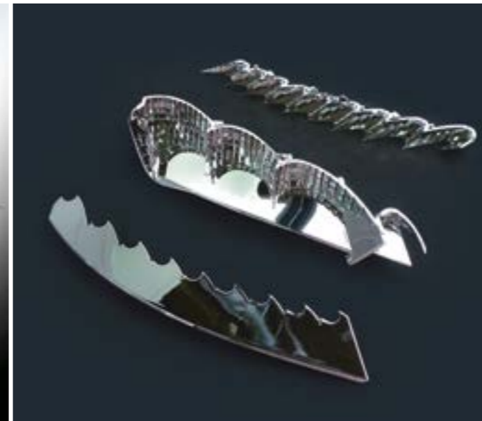
Reflectors from the prototype light after vacuum plating.
