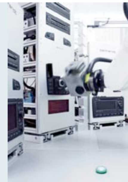
Robots testing infotainment-components.
