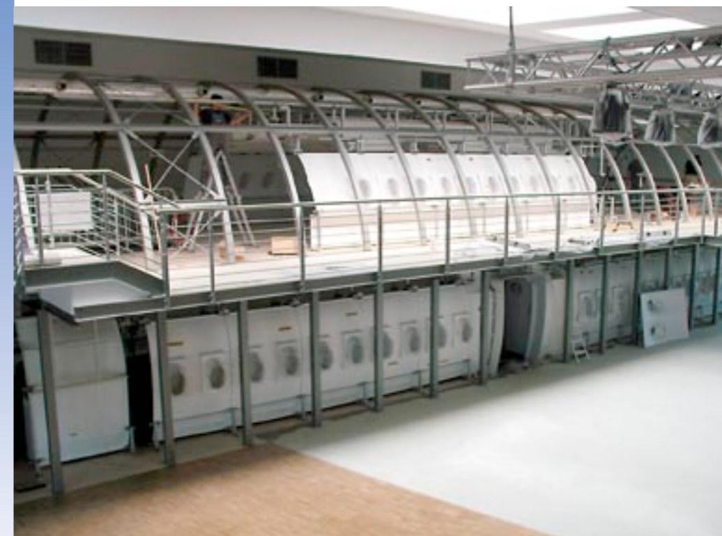
The Cabin System Test Center being assembled. The first interior panel trims are installed.
