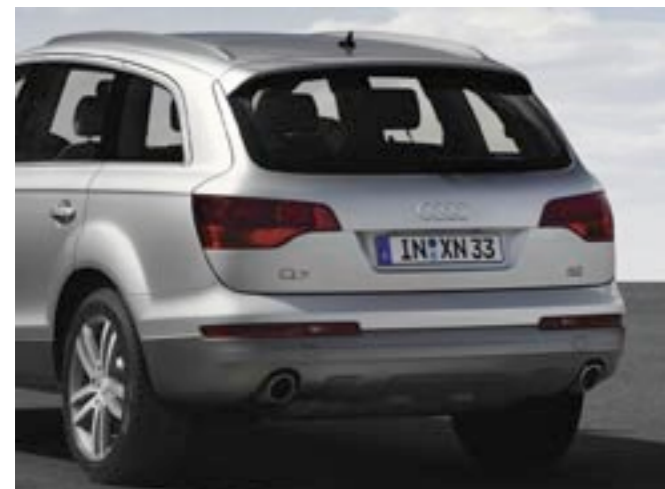
The entire rear light unit is integrated into the rear-hatch.
