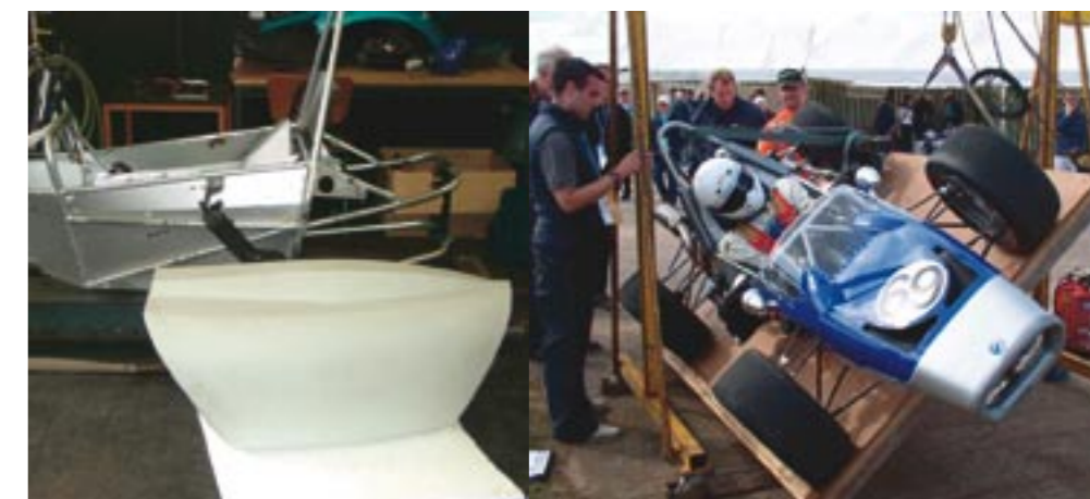
Ureol models of the HAWKS racing team's car from the Hamburg College of Higher Education.
