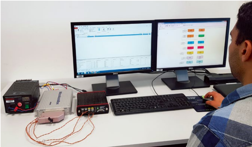
FIGURE 4 Laboratory workplace with MABX2 hardware and development laptop (© Bertrandt)
