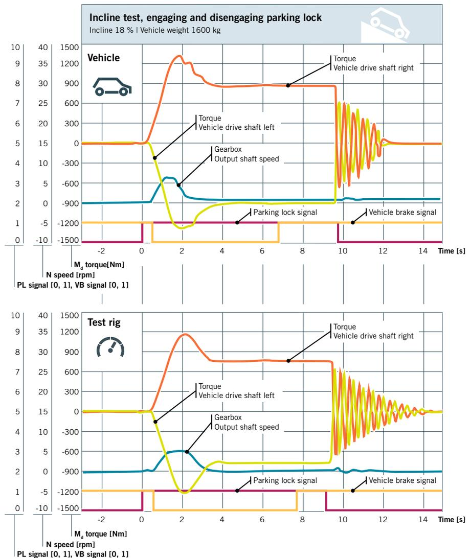
**FIGURE 4** The test shown describes a situation involving parking on a slope and pulling away again (© Bertrandt)
