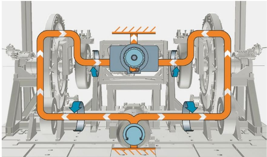
**FIGURE 3** Test rig for gearbox parking locks: When the parking lock is engaged, the test torque applied via the vehicle tires is transferred to the gearbox housing and then via the gearbox mounting points to the test rig, which closes the torque path (© Bertrandt)
