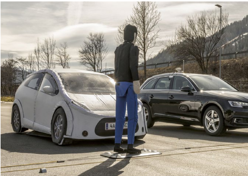
FIGURE 5 Vehicle (C2 target) and pedestrian dummy (adult pedestrian) in combined use (© Bertrandt)
