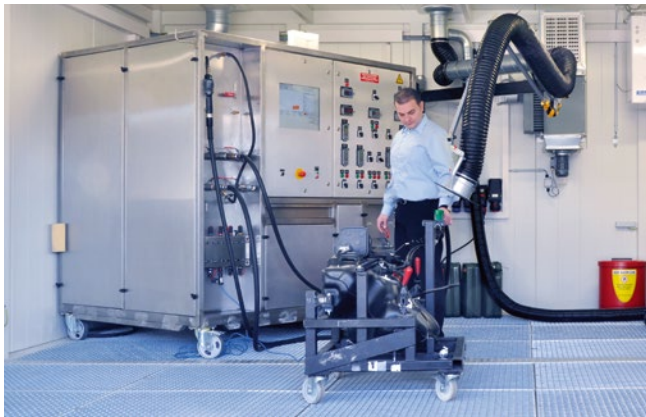
FIGURE 1 Validating the safety and speed of the refuelling process with a test facility (© Bertrandt)
