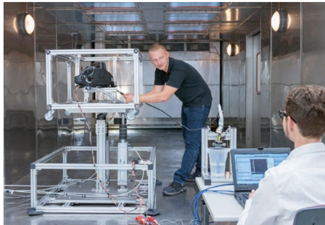
FIGURE 2 Investigating the thawing speed of an SCR system (© Bertrandt)
