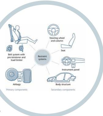
at one of Bertrandt's sites in Germany (Above) The components of a frontal restraint system (Below) The development process for a car's frontal
